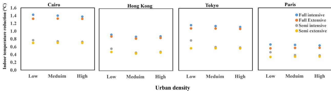
Fig. 8. Indoor temperature reduction under different green-roof types, climates and urban densities.
