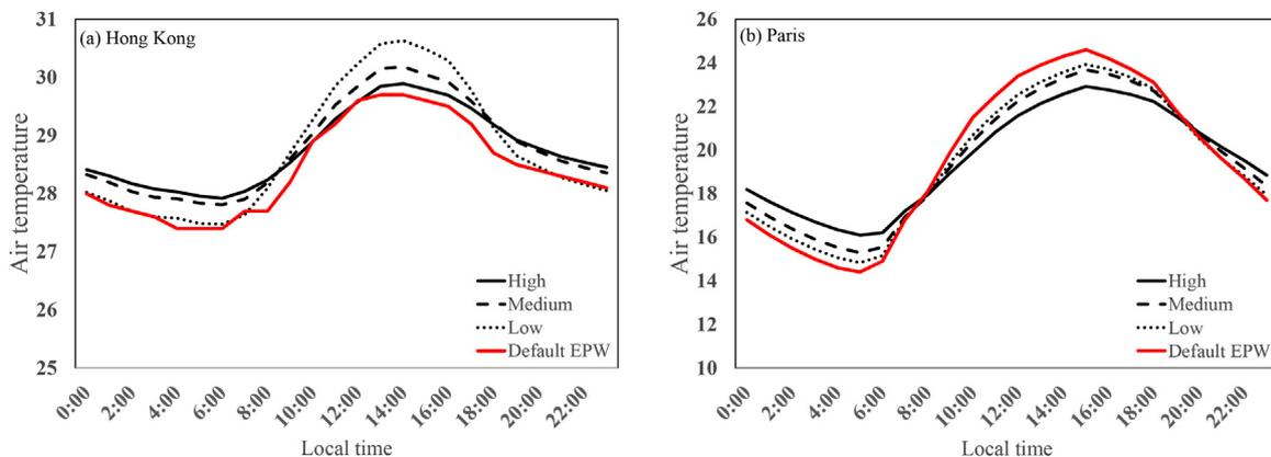
Fig. 3. Comparison between air temperature data in default and modified EPW with different urban densities in (a) Hong Kong and (b) Paris as an illustration.
