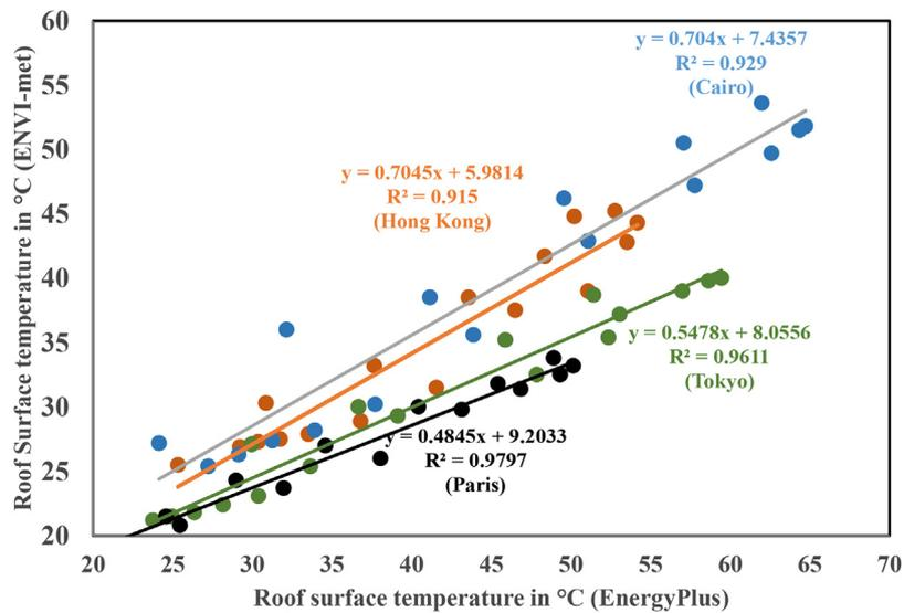
Fig. 6. Relationship between ENVI-met and EnergyPlus simulated hourly roof surface temperature for the four climates.
