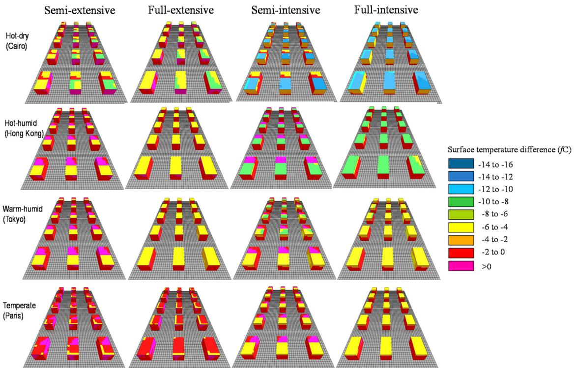
Fig. 7. Effect of green-roof types on roof surface temperature under difference climate at 12:00 noon. This plot is for low urban density and almost similar for High and medium densities.
