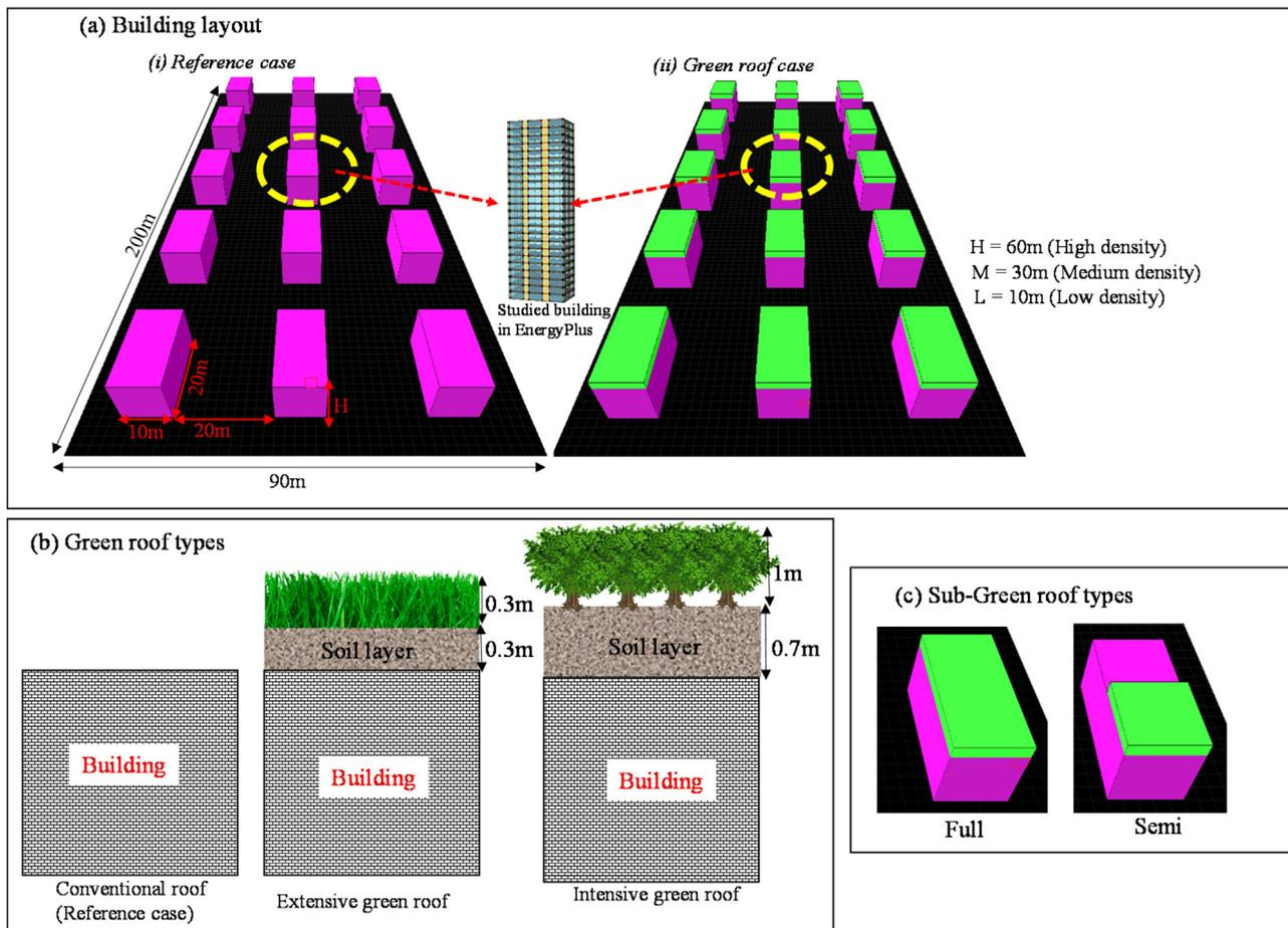
Fig. 1. Schematic diagram of (a) ENVI-met's building/neighborhood layout, (b) green-roof types and (c) sub-green-roof types.
